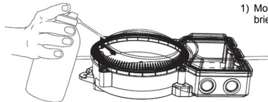
1) Move the "test hole plug" to the side and briefly release a spray of aerosol.
