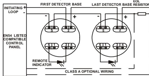
NOTE: IF REMOTE INDICATOR IS NOT USED, POLARITY TO DETECTOR MAY BE REVERSED.
