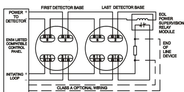
**Fig.1.b. Installing the 4-wire heat detector base**
