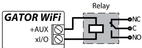
Using the contact of the relay, it is possible to remotely control (turn on/off) various electric devices. The "Output" mode must be set to the **xI/O** terminal.
