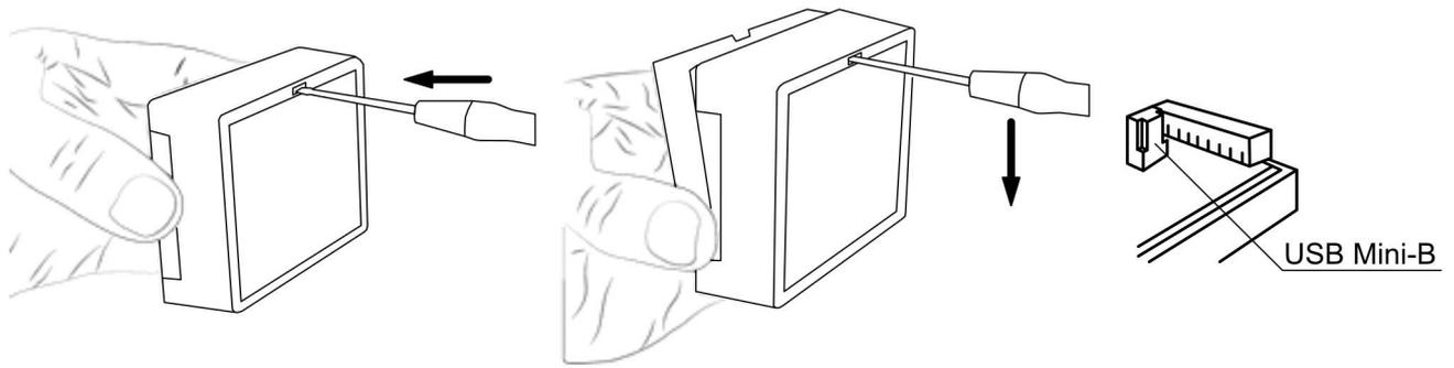
3. Connect the **GATOR WiFi** to a computer using a USB Mini-B cable.
