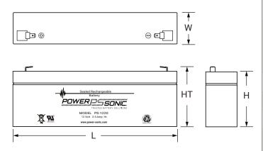
L: 5.28 (134) W: 1.34 (34) H: 2.35 (60) HT: 2.56 (65) Tolerances are +/- 0.04 in. (+/- 1mm) and +/- 0.08 in. (+/- 2mm) for height dimensions. All data subject to change without notice.
