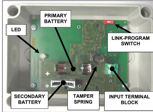
Picture 2 - The PCB of the device
