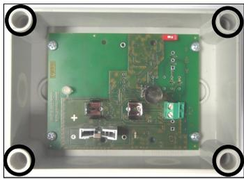
Picture 3 - Wall fixing screw entry points
